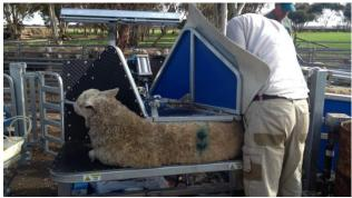
The new sheep handler allows multiple jobs (e.g. crutch, vaccinate, drench, weigh) to be done easily in one quick pass reducing stress on the sheep and the operator
